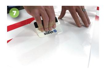
Laying the liner over the graphic with the shiny side facing you, apply hard pressure with the squeegee, removing any stubborn air bubbles.
