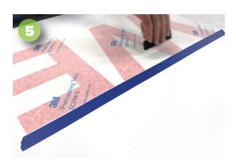
Once in place without creases or bubbles, squeegee the entire lettering or graphic to ensure the adhesive is firmly attached to the surface.
