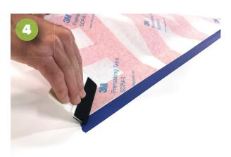
Using a squeegee\*, apply pressure to the front or pre masked side of your lettering, placing the graphic onto the intended surface. Squeegee from left to right from the top down. If creases or bubbles develop, carefully lift the graphic and re-squeegee it.
