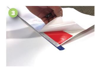
Hold the bottom edge of the hinged graphic away from the intended surface and remove the back liner (which is different from the transfer tape), revealing the sticky backing of your lettering or graphic. Be careful not to allow the exposed adhesive to touch the surface.
