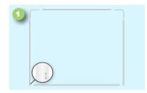
Lay the poles out on the ground in the basic shape of the tension fabric display. Each pole is labeled with a numbered sticker. The numbers will match to show which sides should be connected. Ex. 1 matches with 1, 2 matches with 2, etc.
