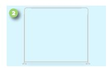
While still on the ground, connect all the poles. The poles use a 'push-button' locking mechanism that secures the poles together. (If it is a straight display, you will need to connect the feet to the poles by screwing them in).
