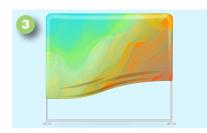
Slide the tension fabric over the now assembled poles.
